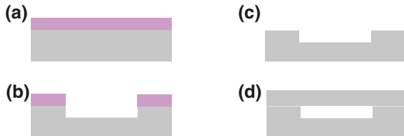
FIG. 8. Schematic of the nanofabrication process steps of nanofluidic geometries. (a) Substrate (gray) is covered with a masking layer (pink) prior to the lithography step, (b) lithography followed by substrate etching, (c) substrate cleaning, and (d) direct wafer bonding.
